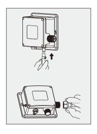
1,Connect flexi hose from faucet to outlet of control box, squeeze clamp over hose and slide pipe onto outlet of control box then release clamp to secure.
