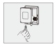
Connect cable with control box, then screw tightly
