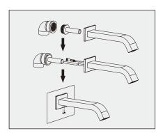
2. Push the sensor cable and flexi hose through the pipe, and fix the faucet body.
