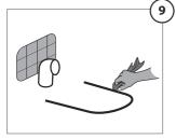
· Apply industrial paste along inside of peripheral outline on floor.
