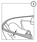
· Measure the thickness of the wall of the foot near to the fixing hole area (t) of the water closet as shown in the figure
