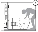
· Place the suit correctly and connect the WC outlet to the drainage pipe
