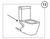
Connect water inlet valve to angle valve.
