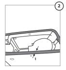
Measure wall thickness of water closet foot near fixing-hole area (t)
