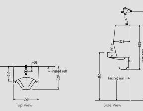
\*\* Approximate measurements for comparison only CONFIGURATION WALL MOUNTED URINAL Weight 20 kg Height - Floor to Rim Nominal Dimensions 650 mm 350 X 320 X 615 mm
