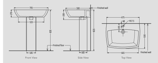
\*\* Approximate measurements for comparison only CONFIGURATION VESSEL/COUNTER TOP 21.5 kg 635 X 345 X 155 mm Weight Basin Area Height - Floor to Rim 850 mm Nominal Dimensions 705 X 500 X 200 mm Faucet Hole 35 mm Waste Hole 45 mm
