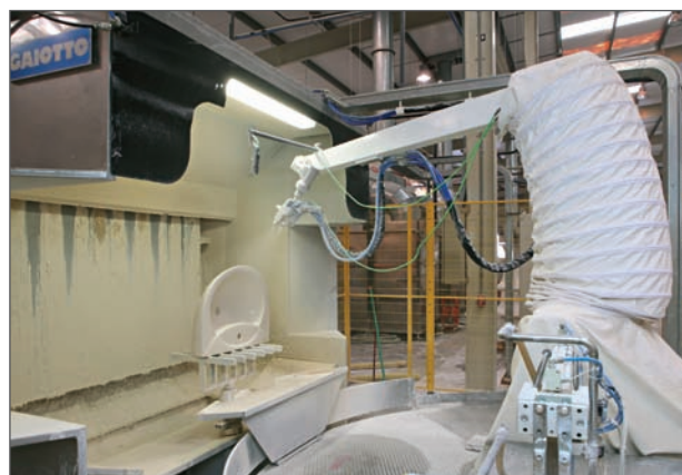
"Robotised Glazing machine in operation"
