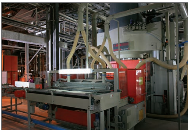
"Largest press-machine in Sri Lanka commercially producing 60cm x 60cm sized tiles"
