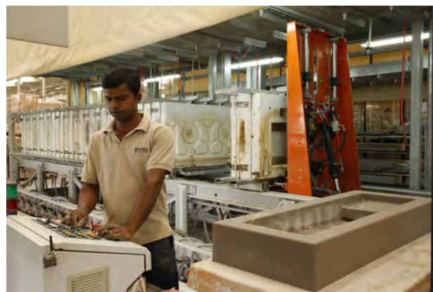
Production of large sized fireclay products at the Rocell Bathware production complex
